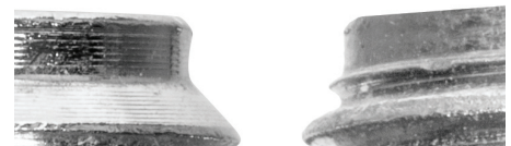
Optimized Thread Relief Standard Thread Relief
